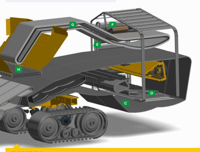
TYPE 75.726 3 sieving webs, star roller separator (8 star rollers), steep pintle belt with air support and a de-viner web
